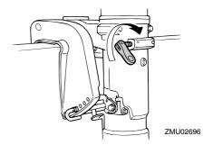
Tighten the air vent screw. On models equipped with a fuel joint, disconnect the fuel line from the outboard motor.
